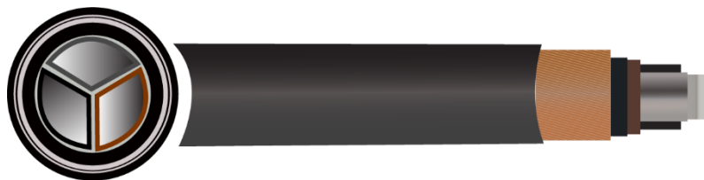
Figure 1 Example of a concentric cable to BS 7870-3.40
