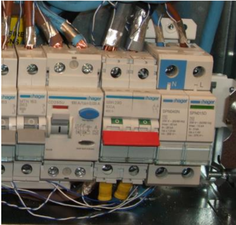
Figure 2 Temperature rise testing thermocouples placed at designated points with SPD adjacent to the main switch. Image reproduced by permission of Hager Group
