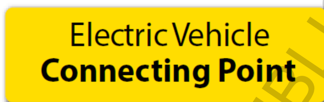
Figure 4.4 4.4 Label for socket-outlets suitable for EV charging
