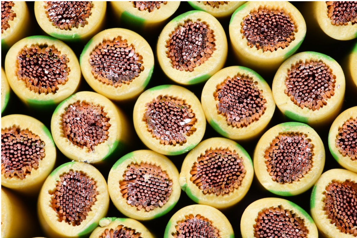
Figure 4: Solid yellow coloured insulation with green stripe
