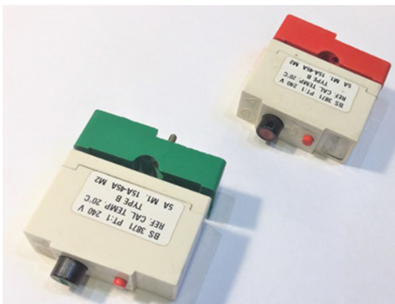
Figure 7 - BS 3871 plug-in miniature circuit breaker of a style produced from the late 1960s to 1985
