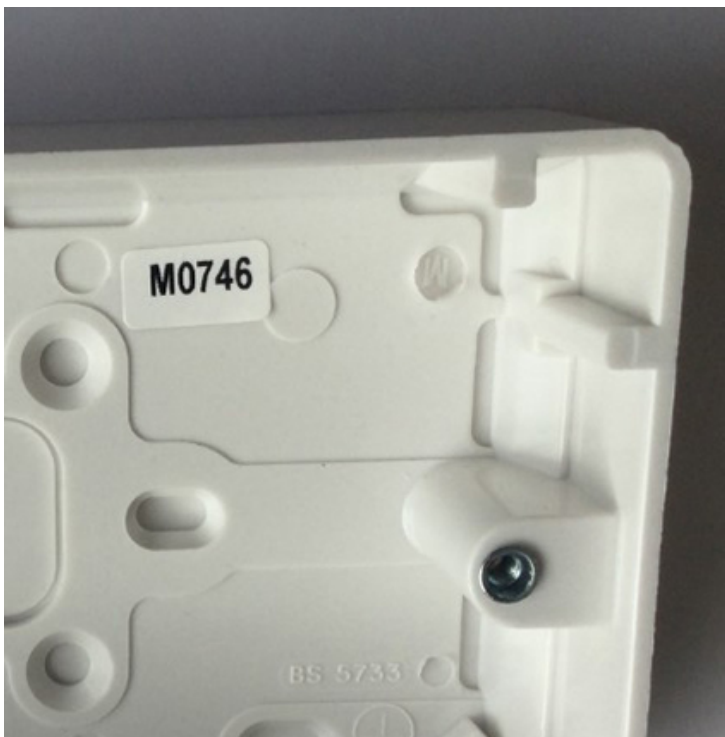
Figure 5 - Date coding on a wiring accessory showing week 46 of 2007
