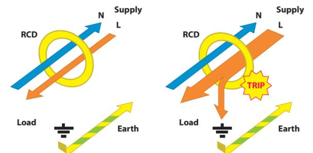
The device monitors the ingoing and outgoing current flow and trips when an imbalance occurs as illustrated above.
