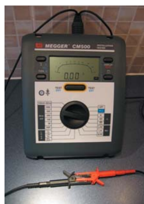
Fig 3: Leads nulled in the incorrect manner
