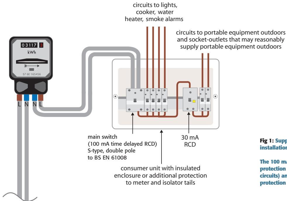
**Fig 1: Supply to a Grade E system where the installation forms part of a TT system.**
