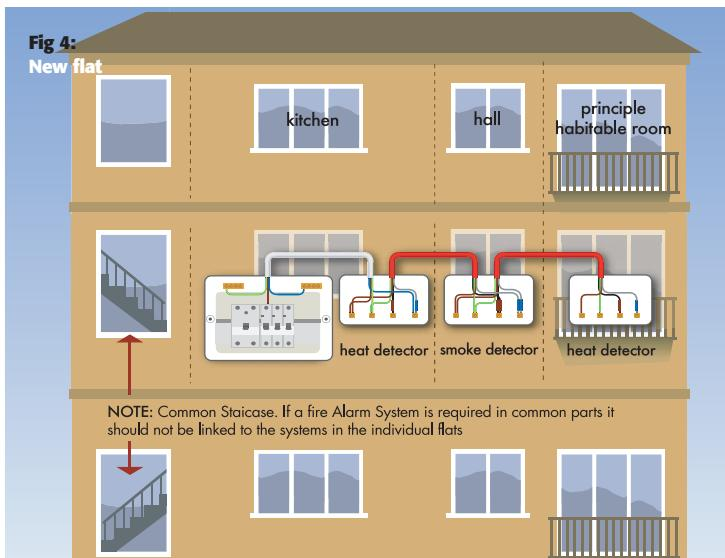
The entire system should be tested to ensure that it operates satisfactorily and that, in particular, automatic fire detectors and any manual call points function correctly when tested. Smoke detectors should be smoke tested with a simulated smoke aerosol that will not damage the detector. Heat detectors should be tested by means of a suitable heat source unless detector damage would otherwise result. The heat source should not have the ability to cause a fire. A live flame should not be used.
