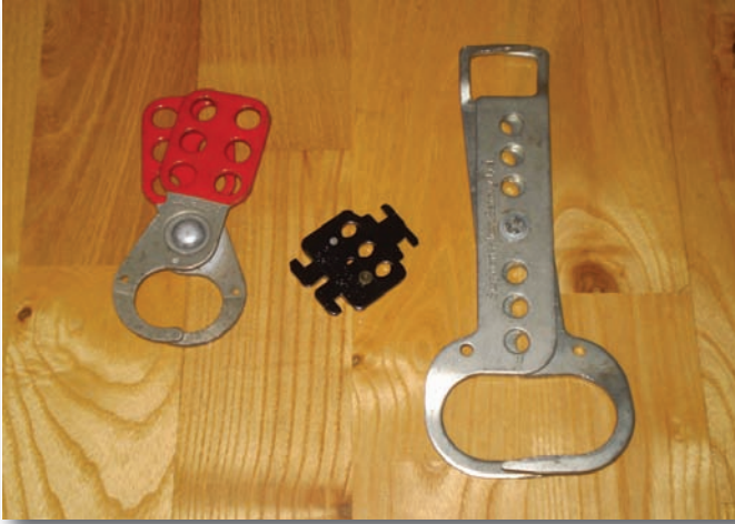
Examples of lock-out devices permitting more than one person to apply a lock for reasons of safety
