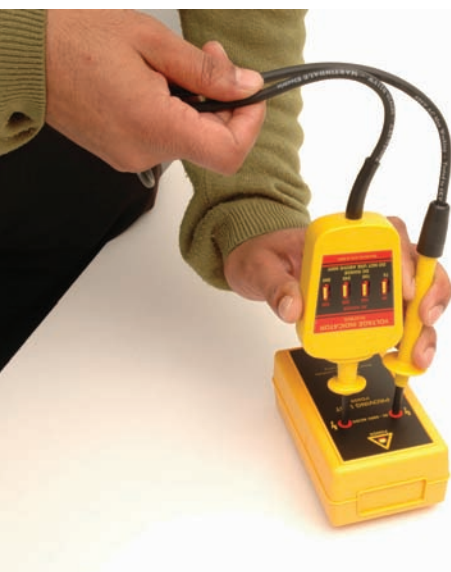
Use of proving unit to verify functionality of voltage indicator
