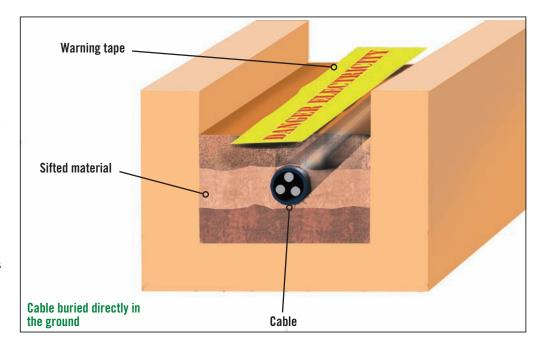
Important: a rating factor has to be applied where the installation conditions differ from those for which values of current-carrying capacity are tabulated in Tables 4D1A to Tables 4J4A of appendix 4.
