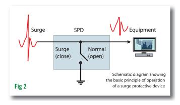
let-through voltage) no more than 1600 V whilst Type 2 and Type 3 SPDs should have a protection level *U*p no more than 600 V when tested in accordance with BS EN 61643 series. Given that transients can be present between all conductors or modes (for example line to earth, line to neutral and neutral to earth) it is important to ensure good protection level *U*p in all such modes.
