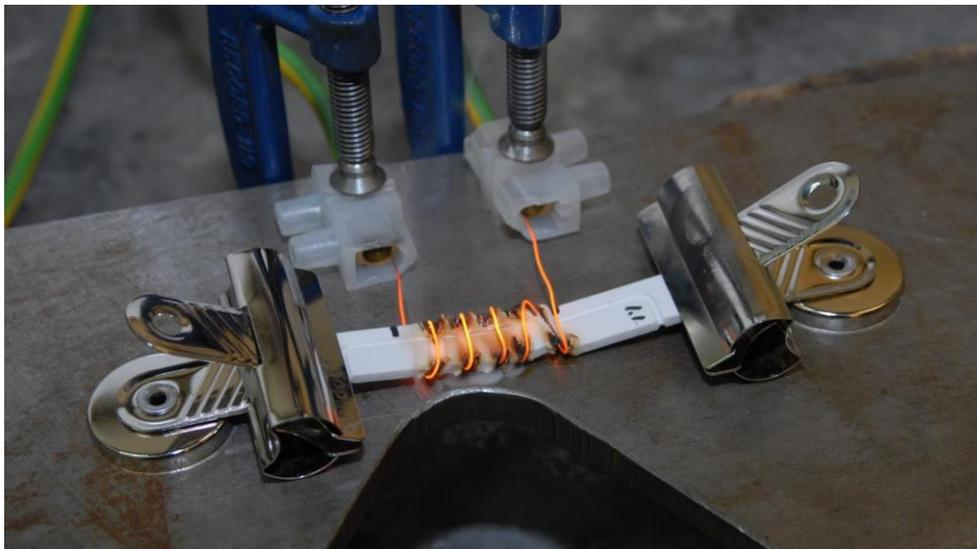
*Testing of a small piece of plastic from a consumer unit with a heated 'hot wire'.*
