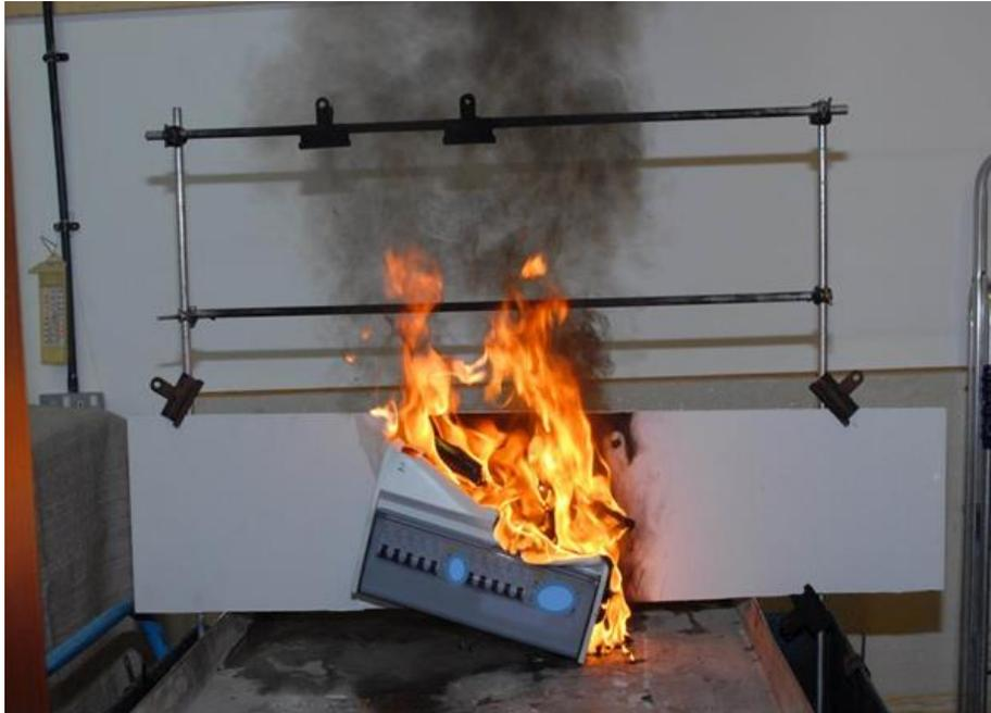
*A consumer unit test in progress - the fire rapidly burnt through mountings causing the test to be stopped.*
