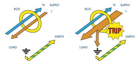
The device monitors the ingoing and outgoing current flow and trips when an imbalance occurs as illustrated above.
