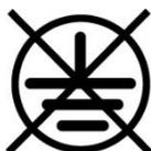
Likewise, equipment having un-insulated live parts must have basic and supplementary insulation provided. If this cannot be achieved it is allowable to use reinforced insulation as long as in doing so a degree of protection not less than class II is provided. Again, a symbol to indicate no earth present must be clearly displayed on the equipment.
