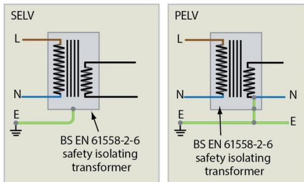
It is for this reason that where a PELV transformer is used and the nominal voltage does not exceed 25V a.c or 60V d.c, in a normally dry location, the exposed conductive parts must be connected by a protective conductor to the main earthing terminal for the installation, where protection against contact with live parts may be omitted.
