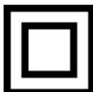
In instances where equipment to be used in this type of system only have basic insulation, the installation must have supplementary protection applied to it during erection, to provide a measure of safety no less than that of class II equipment. The equipment must also be clearly marked with a symbol to indicate there is no earth present, see below:
