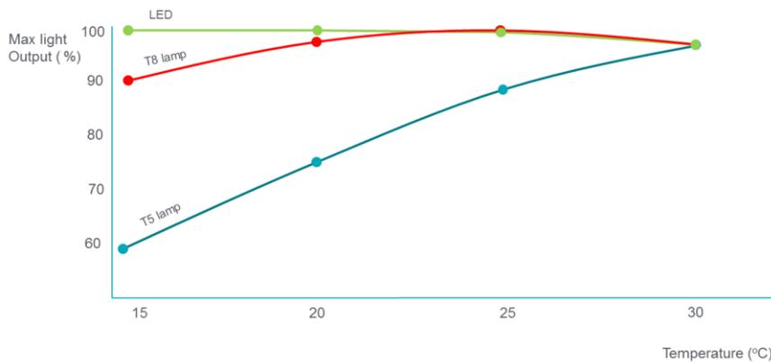
It can be seen that the output of the T5 lamps is affected to a greater extent than T8 or LED when the temperature around the lamp falls. If integrated cooling/lighting solutions are not properly designed, there could be a noticeable difference in illumination levels depending on whether the mechanical systems are cooling the space at any given time.
