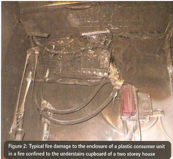
Figure 2: Typical fire damage to the enclosure of a plastic consumer unit in a fire confined to the understairs cupboard of a two storey house
