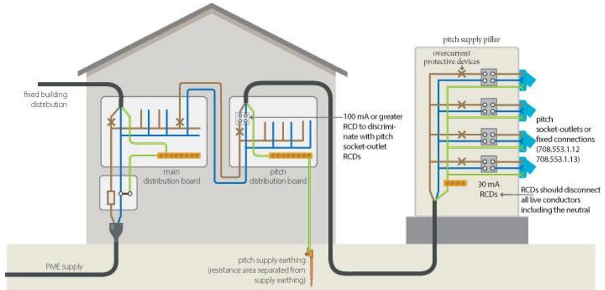
Alternatively, the separation of the earthing can be made at the caravan pitch supply points. In this instance, earth electrodes will be required at these points. See the below Figure 7.2 of IET Guidance Note 7 for detailed information.
