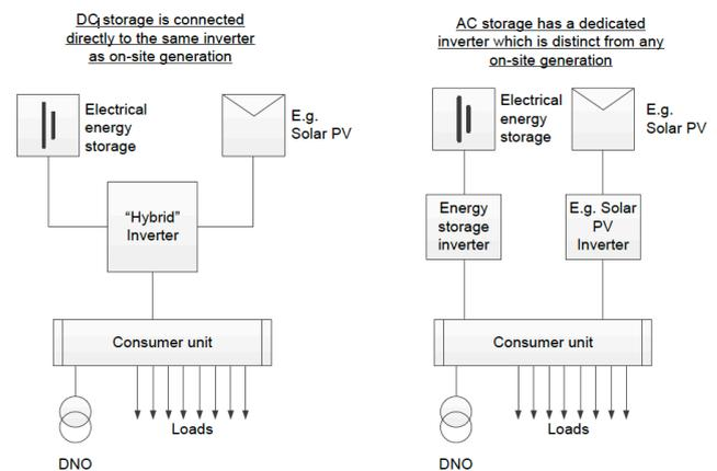
Figure 1: DC- and AC-connected energy storage
