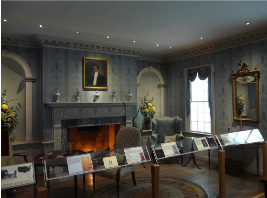
*The American Museum in Britain, lit with eighteen 2 W adjustable LED downlights. These were positioned on the ceiling to light a given area or object well with a specific beam angle. For example, the long information panel at the front was lit by just three spots with elongation beams to give a long wide light spread.*
