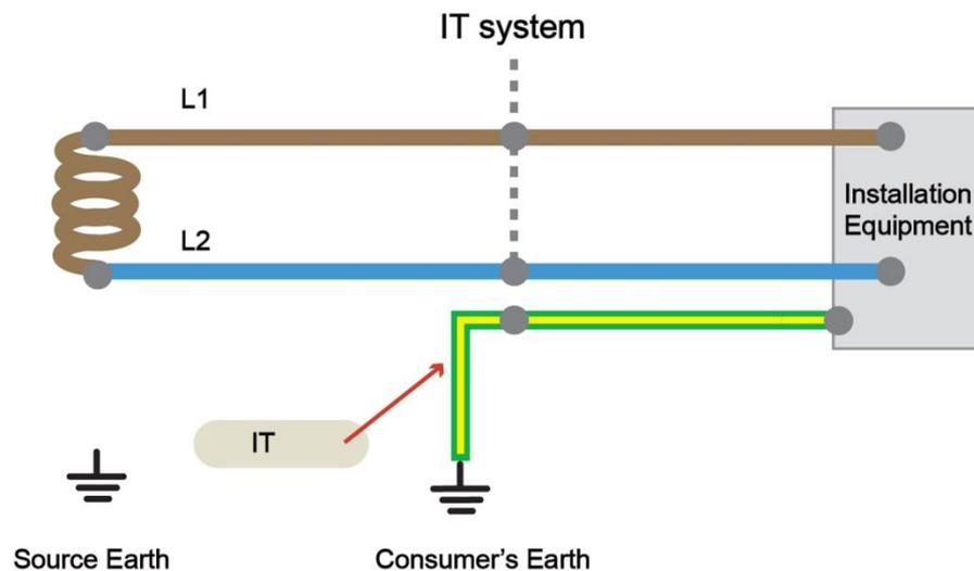
It is worth noting the colour scheme shown in the diagram above, in particular the fact that both cores are live so there is no neutral. The two live cores are usually referred to as L1 and L2 even though the system is effectively a single-phase system; due to this, and to ease identification, Network Rail use brown and black for L1 and L2 respectively.
