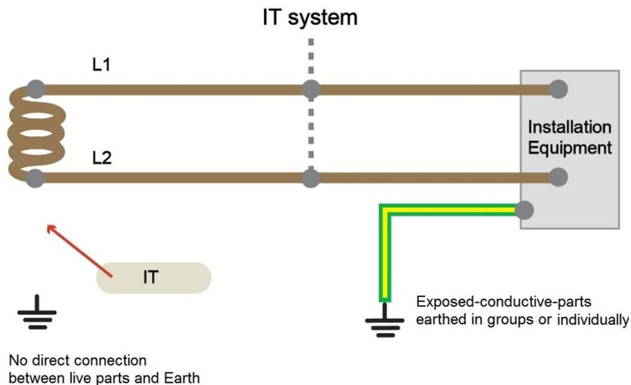
The third type of earthing arrangement, and the particular focus of this article, is the 'IT' type, in which the source transformer is isolated from earth, whilst all exposed conductive parts of the installation are connected to earth electrodes. So what are the benefits and where are IT systems used? To answer these questions it's best to first look at how the system operates, especially in a fault situation.
