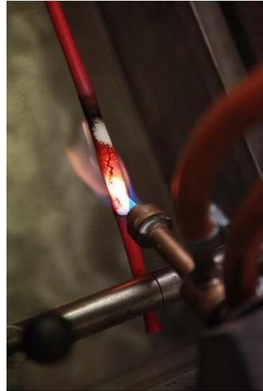
*The Bunsen burner flame propagation test*
