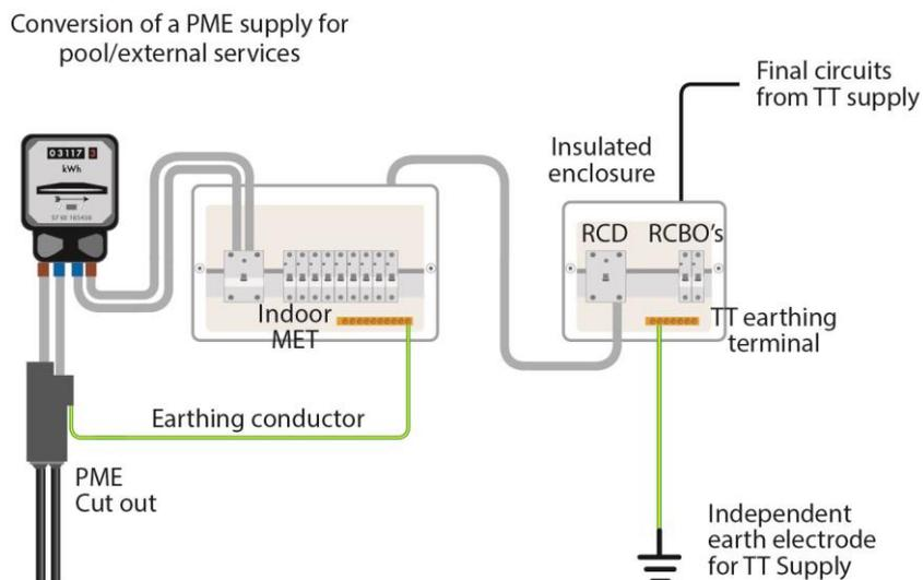
Once the TT arrangement has been formed with the appropriate earth electrode it is necessary to ensure that this system and any of the pool extraneous-conductive-parts are not connected to the PME earthing system by any 'casual' connection, as this would only serve to create problems.
