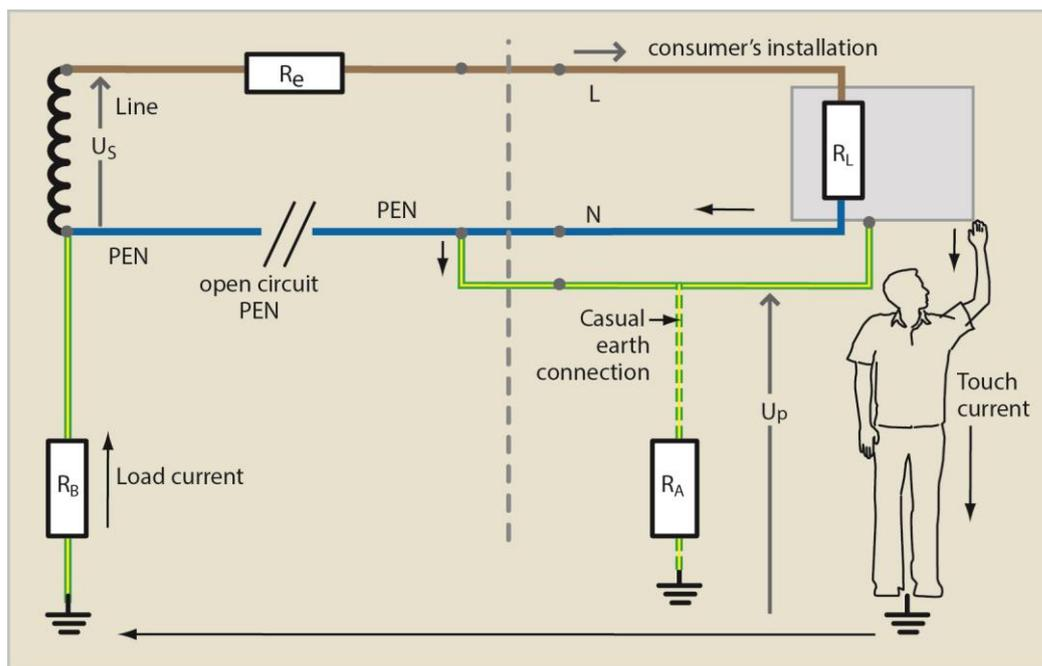
The touch voltage will be determined by the load connected within the installation and the value of the earth electrodes and any casual connections to earth that is provided by the bonded services.
