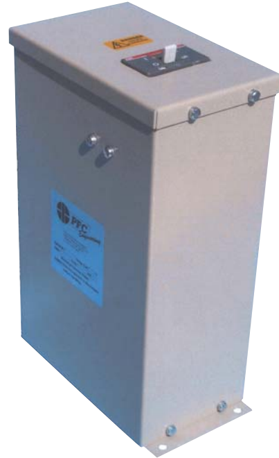
Capacitor module designed for local correction of individual loads such as single motors, starters or control gear incorporating an integral circuit breaker for independent isolation and overload protection.
