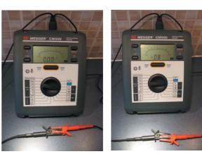
Fig 3: Leads nulled in the incorrect manner
