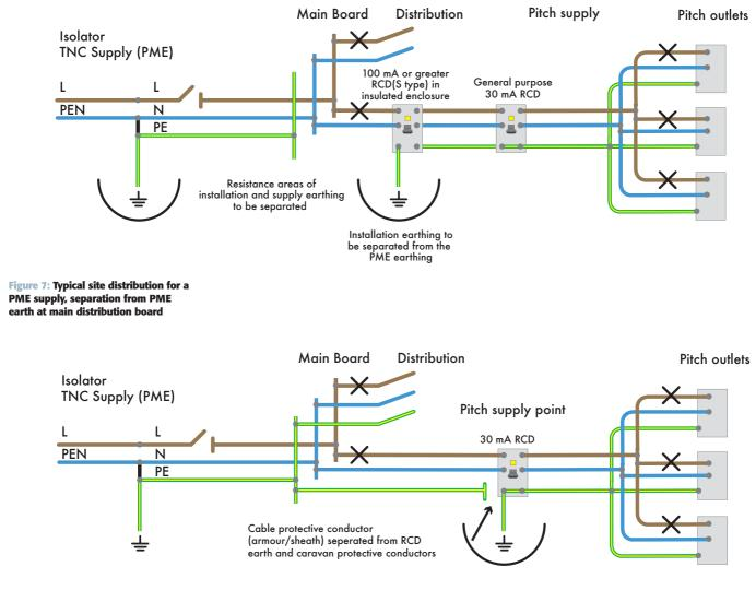
Figure 8: Typical site distribution for a PME supply, separation from PME earth at pitch supply point
