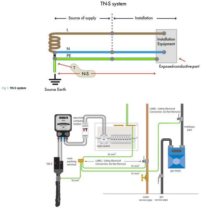
Fig 2: Cable sheath earth (TN-S system). Schematic of earthing and main equipotential bonding arrangements. Based on 25 mm<sup>2</sup> tails and selection from Table 54G. Note: An isolator is not always installed by the electricity distributor.
