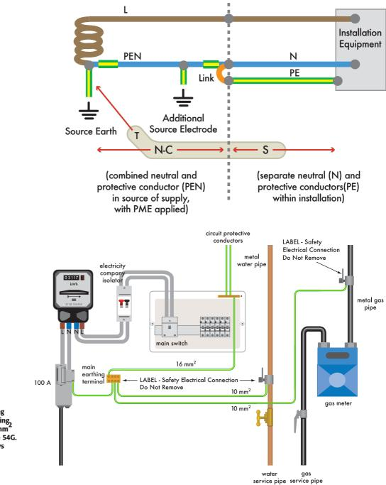
Fig 4: PME supply (TN-C-S system). Schematic of earthing and main equipotential bonding arrangements. Based on 25 mm<sup>2</sup> tails and selection from Table 54G. Note: An isolator is not always installed by the electricity distributor.
