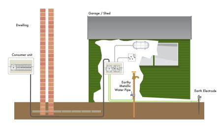
Fig 3: Garage installation made part of a TT system
