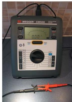
**Fig 3: Leads nulled in the incorrect manner**
