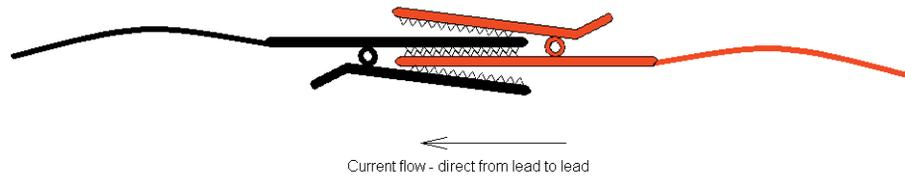
**Fig 1: Correct method of connection**
