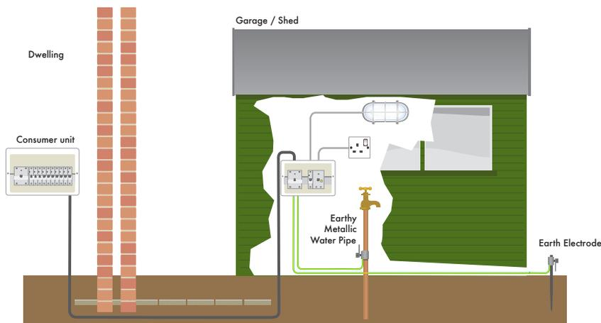
Fig 3: Garage installation made part of a TT system
