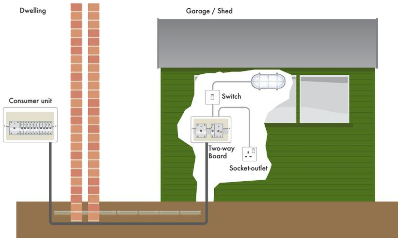
**Fig 1: Garage supply taken from a spare way in the consumer unit**
