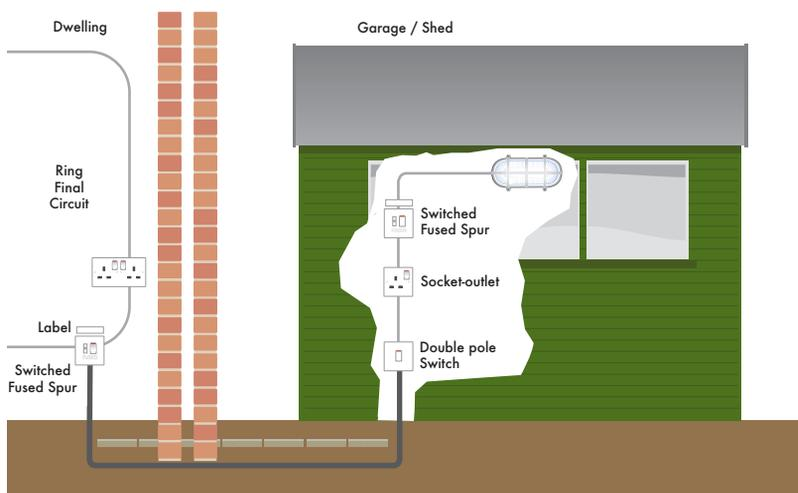
**Fig 2: Garage supply taken from a spur off the downstairs ring final circuit**
