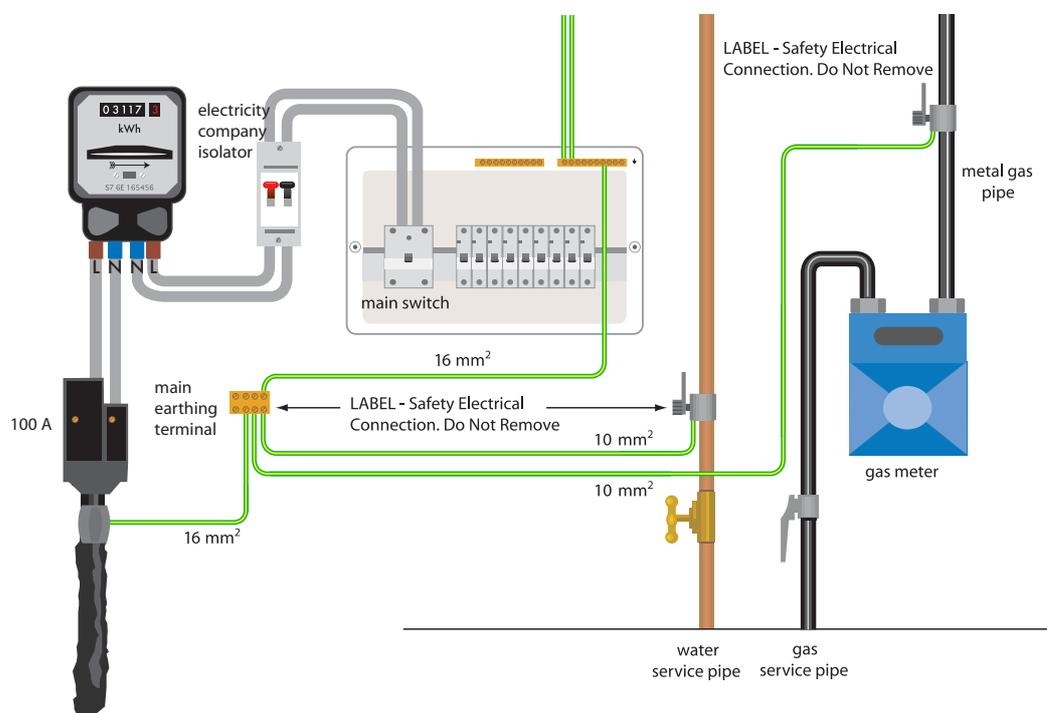
Fig 2: Cable sheath earth (TN-S system). Schematic of earthing and main equipotential bonding arrangements. Based on 25 mm<sup>2</sup> tails and selection from Table 54G.
