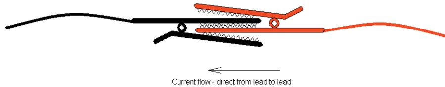
**Fig 1: Correct method of connection**
