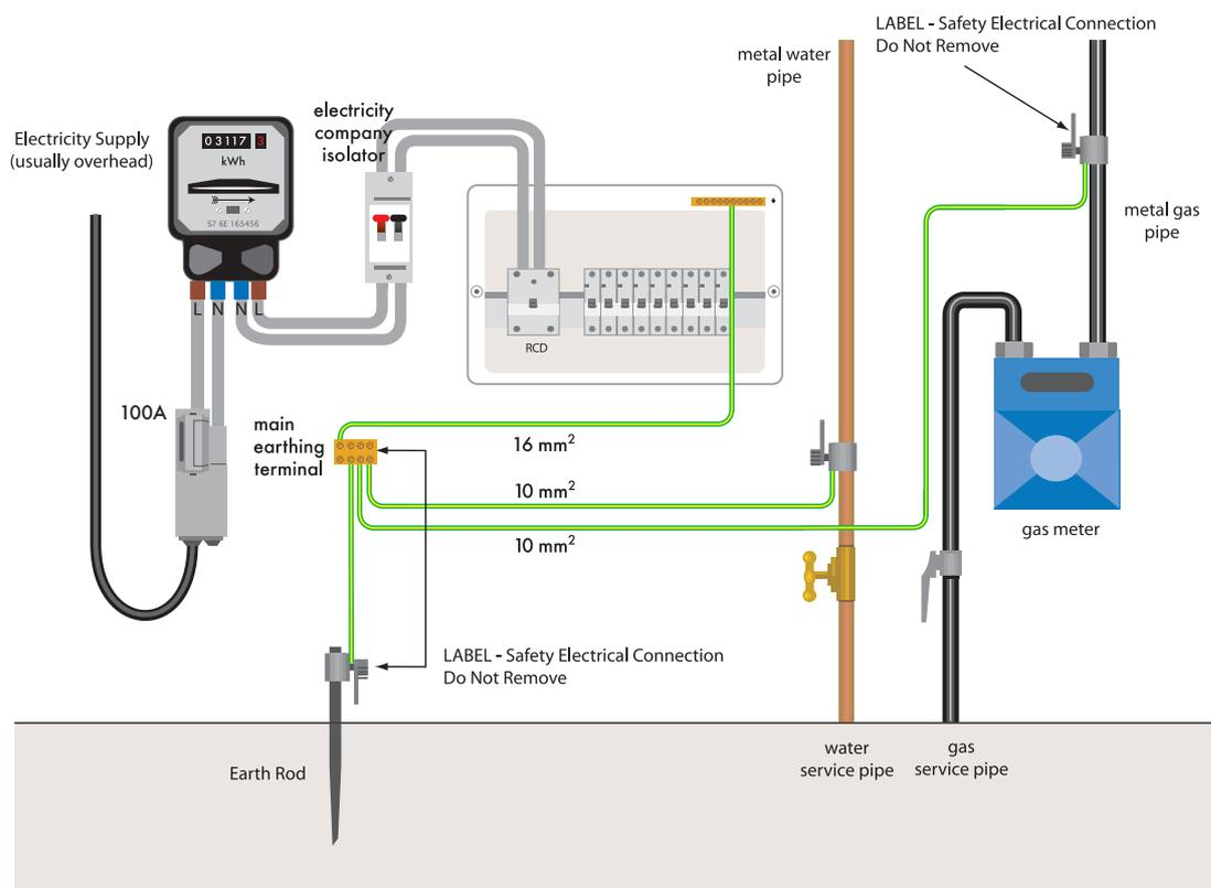
Figure 6: No earth provided (TT system). Based on 25 mm<sup>2</sup> tails and selection from Table 54G. Note: An isolator is not always installed by the electricity distributor. Manufacturers recommendations should be sought with regards to connections to earth electrodes.
