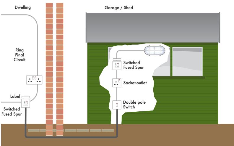
**Fig 2: Garage supply taken from a spur off the downstairs ring final circuit**
