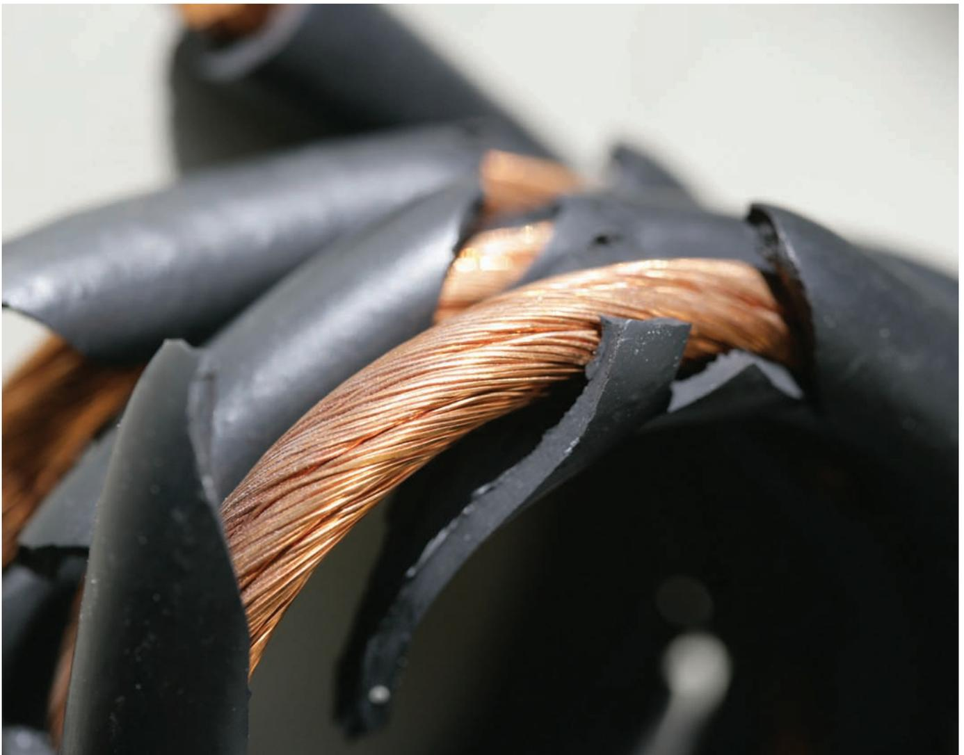
Damaged insulation could have a very serious impact on the unsuspecting engineer. Image courtesy of the ACI
