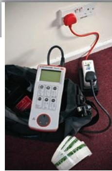
The latest addition to Seaward's range of PAT equipment is the PrimeTest 250. The new hand held PAT provides all the tests required for compliance with the IEE Code of Practice. Special additional test capabilities include an RCD trip time test, a 3-phase leakage test and a 250V DC insulation test suitable for testing sensitive electrical appliances and surge protected leads.
