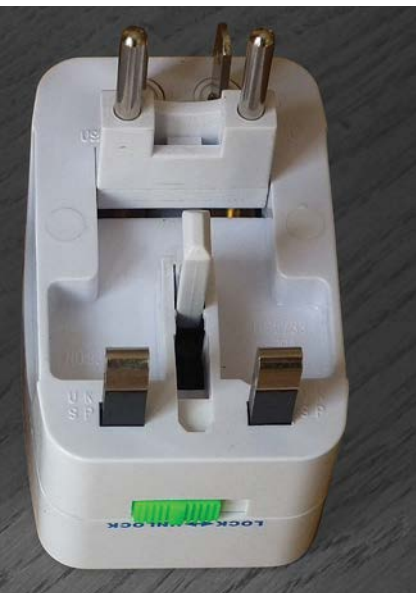
Fig 4 Illegal fusesless plug - a Chinese plug with no provision for a fuse, and the pins set too close to the periphery
