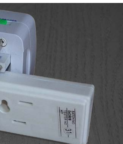
Fig 7 Travel adaptor plugged into socket with live pins exposed to touch, the top (US) pins are spring loaded and can be deployed by releasing the green catch, even after plugging in the adaptor
