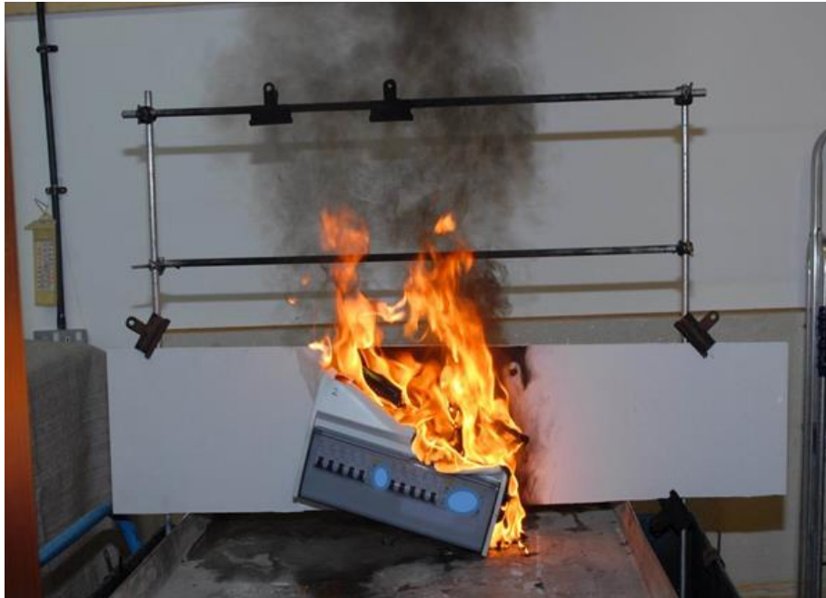
A consumer unit test in progress - the fire rapidly burnt through mountings causing the test to be stopped.
