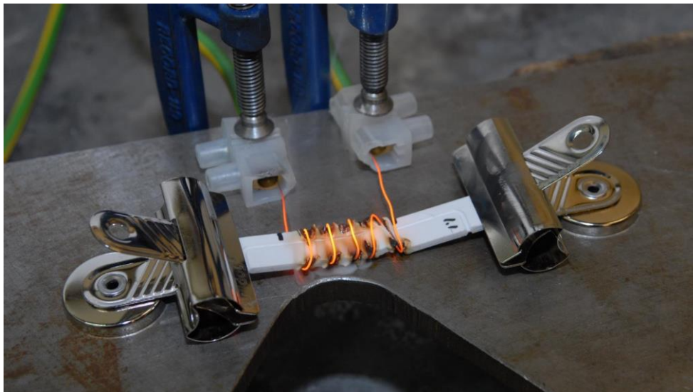
Testing of a small piece of plastic from a consumer unit with a heated 'hot wire'.
