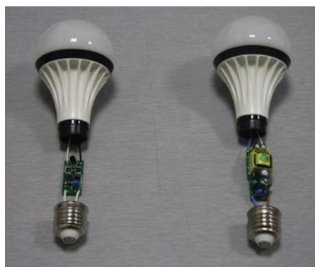
A greatly reduced component count is one major advantage of the ACRE LED (left)
