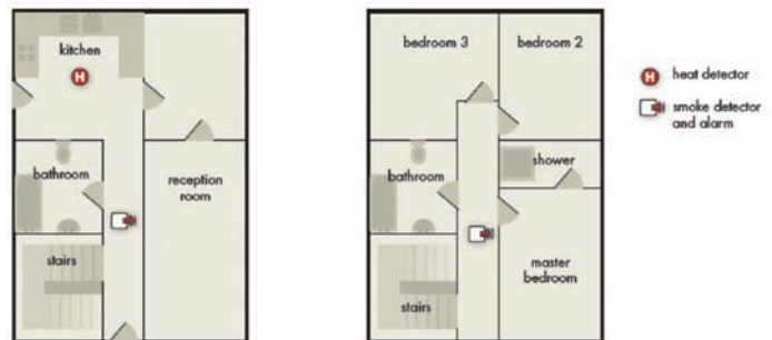
Figure 1: Minimum requirements for smoke alarms (standard house, no storey exceeds 200 m 2 floor area) with the kitchen not separated from the circulation space by a door
